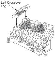
Figure 18 - Installing Left Crossover Log
